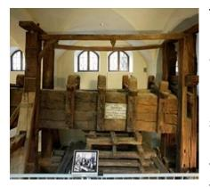
This big wooden winepress originally comes from Metz (France) or thereabouts and was modelled on an ancient paragon. The press exerts controlled pressure in order to free the juice from the grapes. Its pressure is applied through the construction of a lead screw at the end of the press, which is linked to a lever that has to be pressed down onto a basket filled with crushed grapes. By spinning up the lead screw, the lever (made of a whole tree) is forced down on
